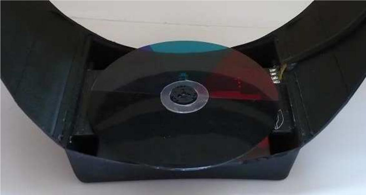
**Fig. 3** View inside the 3d Imager, showing the colour wheel and placement of so called “calibration” wheel/ring.
